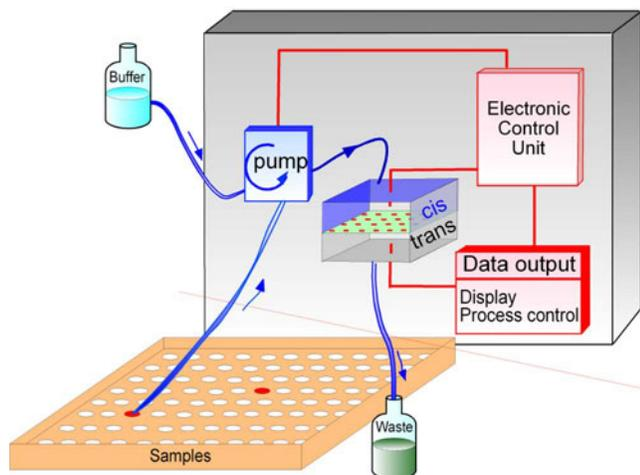
FIG. 6. Scheme of a microfluidic system for monitoring the function of membrane proteins in drug screening.
