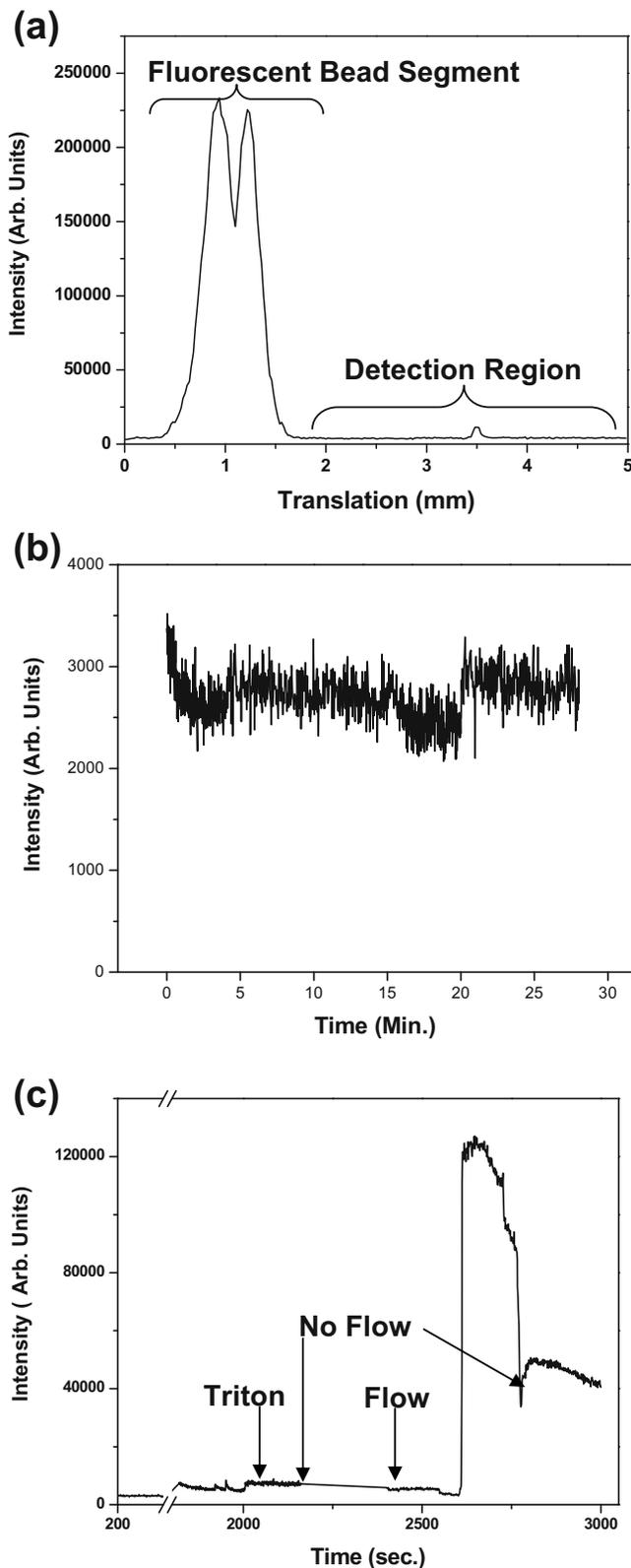
FIG. 9. Stability and Triton X-100 disruption of SLBs in microfluidic studies. (a) Alignment of the microsphere packed microcolumn for fluorimetry experiments. (b) Microfluidic stability study. The very low intensity indicates the stability of lipid-coated microspheres when packed in the microcolumn. (c) Microfluidic disruption upon introduction of 10% (*w/v*) Triton X-100. This figure is representative of three replicates.
