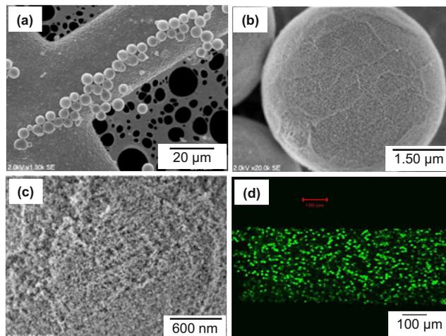
Fig. 1. Images of porous microspheres. (a) SEM image of porous silica microspheres (average diameter=5  $\mu\text{m}$ ). (b) High resolution SEM image of a porous silica microsphere surface. (c) Higher resolution image of a porous silica microsphere showing its porous surface. (d) Confocal fluorescence image of microspheres containing fluorescein encapsulated in lipid bilayer membranes packed in a microcolumn.
