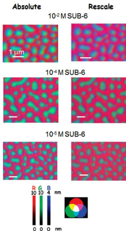
FIG. 4. Color-coded component maps (left, absolute; right, rescaled) for a PS/PMMA blend exposed for 20 min to three different concentrations of SUB-6—(top) 1 \times 10^{-2} mg/ml, (middle) 1 \times 10^{-4} mg/ml, and (bottom) 1 \times 10^{-5} mg/ml.
