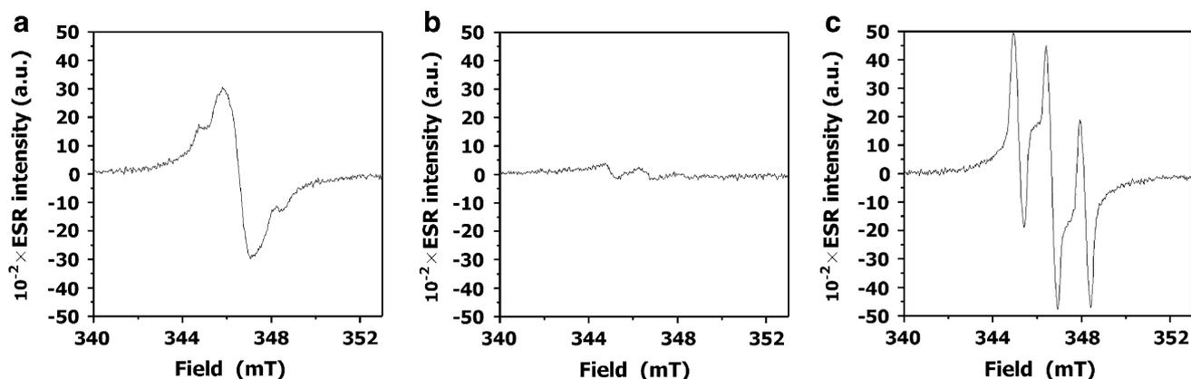
**Fig. 3** ESR spectra of nitroxide radical of RNP (a), HANP (b) after dialysis and disintegrated RNP at pH 5.6 (c) at the same polymer concentration
