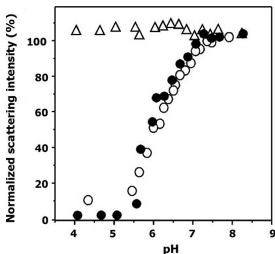
**Fig. 4** Effect of pH on the light scattering intensity of HANP (closed circle), RNP (open circle) and CNP (open triangle). The normalized scattering intensity (%) is expressed as the value relative to that at pH 8.2
