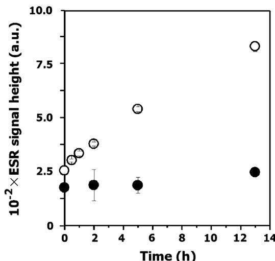
**Fig. 5** Time course of ESR signal height of HANP (closed circle) and TEMPOL-H (open circle) under atmospheric conditions
