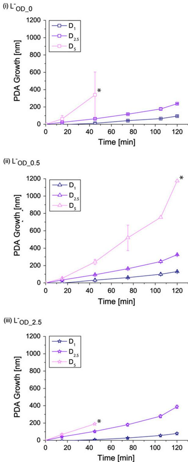
**Fig. 3** Time-course of the normalized increase in diameter for the PDA assembly on negatively charged liposomes with three different amounts of OD [(i) 0, (ii) 0.5 and (iii) 2.5 wt%] using three different concentrations of dopamine (1, 2.5 and 5 mg/mL). The asterisks indicates samples with a PD > 0.4
