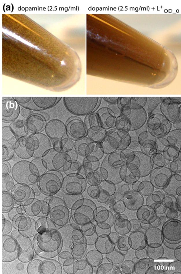
**Fig. 5** **a** Photographs of solutions containing 2.5 mg/mL dopamine in TRIS<sup>1</sup> (left) or 2.5 mg/mL dopamine and L<sup>+</sup><sub>OD\_0</sub> in TRIS<sup>1</sup> (right) after 75 min, showing a flocculated (left) and a homogenous (right) dark brown solution, respectively. **b** Cryo-TEM image of L<sup>+</sup><sub>OD\_0</sub>D<sub>1</sub> showing structurally intact liposomes
