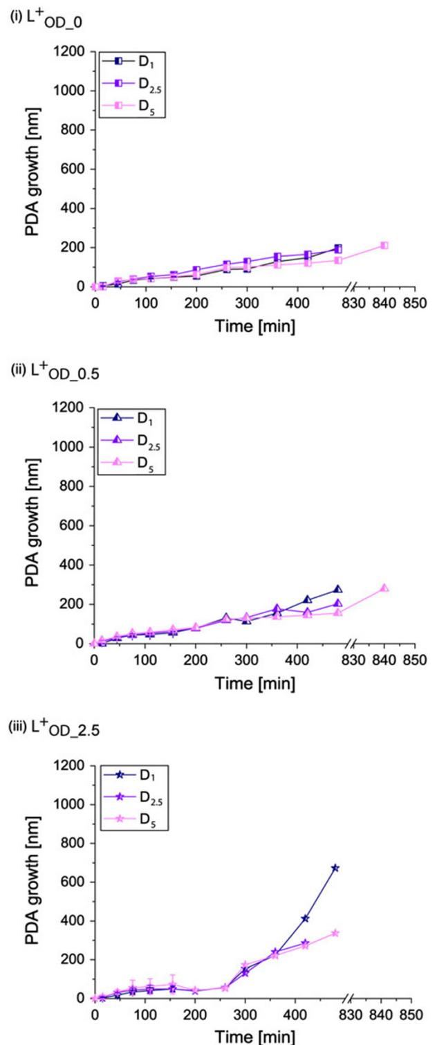
**Fig. 4** Time-course of the normalized increase in diameter for the PDA assembly on positively charged liposomes with three different amounts of OD [(i) 0, (ii) 0.5 and (iii) 2.5 wt%] using three different concentrations of dopamine (1, 2.5 and 5 mg/mL)
