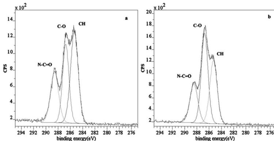
FIG. 3. High resolution C 1s scans of (a) TiO<sub>2</sub> coated Si wafer with adsorbed mucin and (b) TiO<sub>2</sub> coated Si wafer with adsorbed mucin and adsorbed PEG-(DOPA)<sub>4</sub>.
