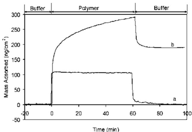
FIG. 5. OWLS traces showing mass adsorbed vs time for interaction of a solution containing (a) PEG-(NH<sub>2</sub>)<sub>4</sub> and (b) PEG-(DOPA)<sub>4</sub> with a mucin coated TiO<sub>2</sub> waveguide. The polymer solution concentration in both cases was 10 mg/mL in 10 mM HEPES, pH of 7.4.
