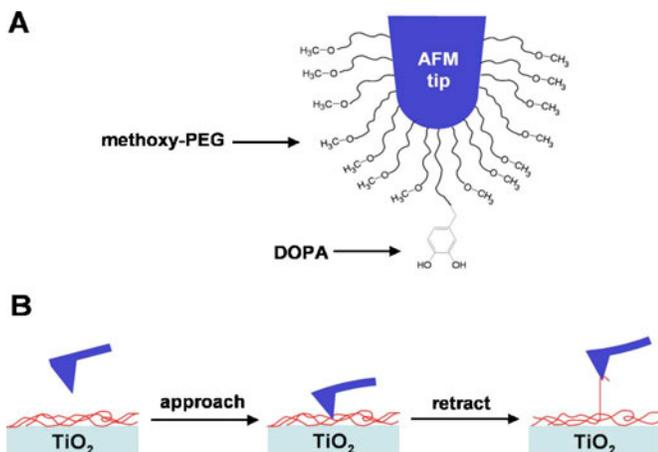
FIG. 8. Schematic illustration of DOPA-mucin AFM experiment. (A) Representation of a covalently modified AFM tip showing a DOPA functionalized PEG chain amidst an excess of methoxy terminated PEG. (B)  $F$ - $D$  curves were obtained by approach of modified AFM tips to a mucin coated  $\text{TiO}_2$  substrate followed by retraction away from the surface.
