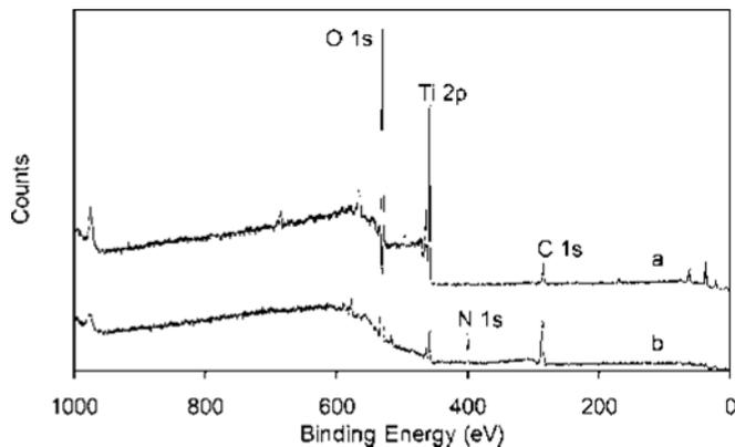
FIG. 2. XPS survey scans of (a) TiO<sub>2</sub> coated Si wafer and (b) TiO<sub>2</sub> coated Si wafer with adsorbed mucin.
