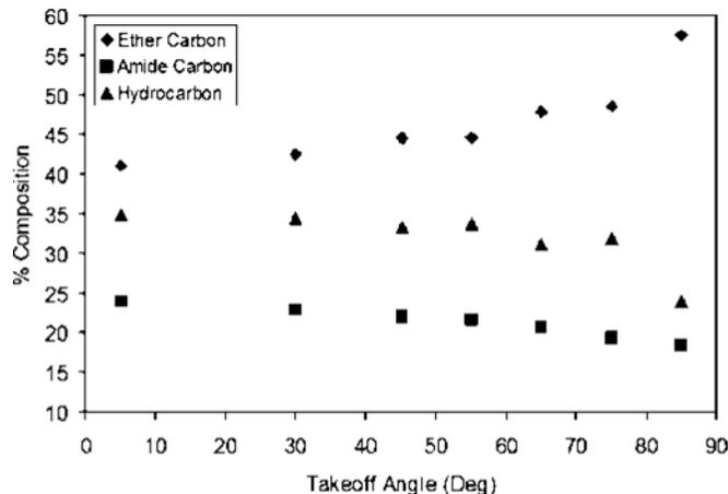
FIG. 4. Percent composition of XPS C 1s peak components vs takeoff angle for the case of PEG-(DOPA)<sub>4</sub> adsorbed to a mucin layer on a TiO<sub>2</sub> coated Si wafer.
