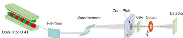
FIG. 2. Schematic overview of the BESSY II STXM (see text) (Ref. 18).
