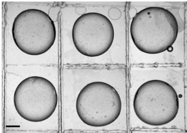
FIG. 2. Positioning 1  $\mu\text{l}$  drops of cell suspension within a  $2 \times 2 \text{ mm}^2$  grid immersed in mineral oil. Scale bar=500  $\mu\text{m}$ .
