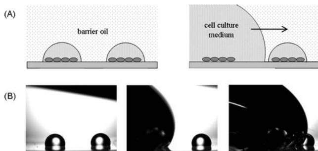
FIG. 1. (a) Schematic of the cell positioning technique. Drops of cell solution are deposited under barrier oil at the desired locations on the substrate. After cell attachment, the barrier oil is displaced by cell culture media, leaving the cells to grow freely from their seeding position. (b) Sequential photos of the displacement process.
