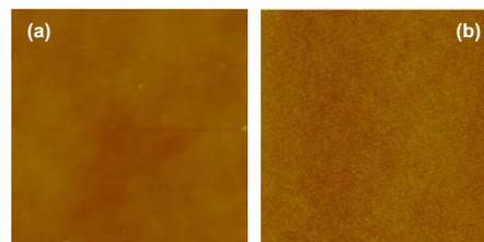
FIG. 1. (Color online) AFM images of initiator-functionalized surfaces: (a) 5  $\times$  5  $\mu\text{m}^2$  image of a film formed from CMPTS; (b) 10  $\times$  10  $\mu\text{m}^2$  image of a film formed from 3-(2-bromoisobutyramido)propyl-triethoxysilane. Vertical contrast range: 0–10 nm in both images.
