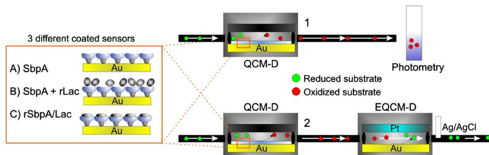
FIG. 1. (Color online) Experimental setup for the determination of the enzymatic activity on QCM-D crystals either by photometry (1) or amperometry (2) on SbpA (a), SbpA and chemically bound rLac (b), and rSbpA/Lac (c).
