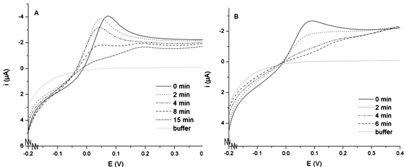
FIG. 4. Voltammograms of HQ at 40 °C and pH 7.7 after the addition of rSbpA/Lac (a) and rLac (b). The applied sweep rate was 10 mV s<sup>-1</sup> in the potential range of -0.2–0.4 V.
