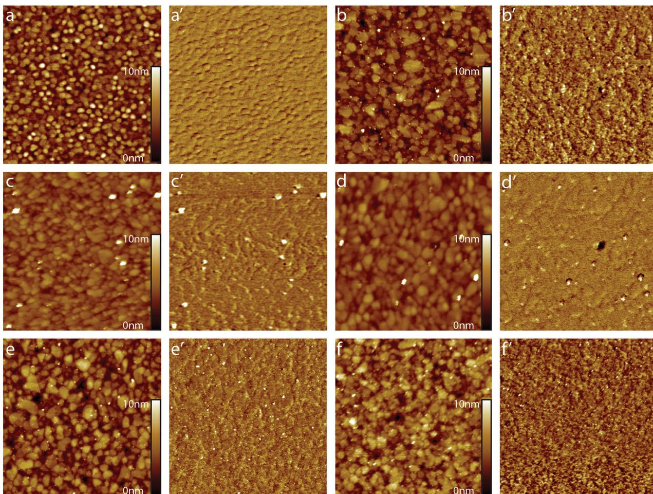
FIG. 3. (Color) Topography and Young's modulus images recorded by QNM-AFM measurements in MQ water. (a), (a') Au substrate. (b), (b') PEG-COOH-SAM. (c), (c') OEG<sub>3</sub>-SAM. (d), (d') R<sub>SAM</sub>. (e), (e') PEG-COOH<sub>SAM</sub> + OEG<sub>3</sub>. (f), (f') PEG-COOH<sub>SAM</sub> + R. The scan area of each image is 1 μm × 1 μm.
