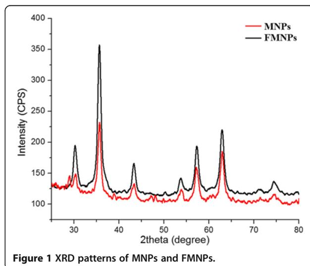
Figure 1 XRD patterns of MNPs and FMNPs.
