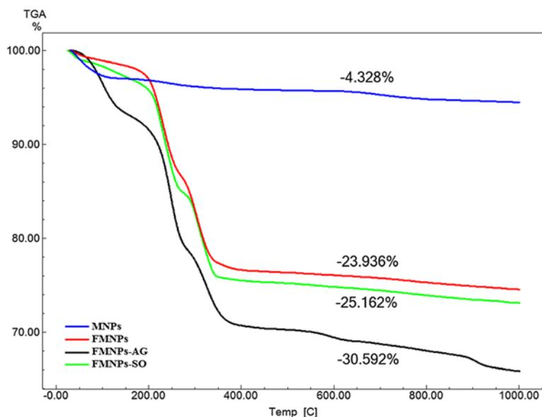
**Figure 3** TGA analysis of MNPs, FMNPs, FMNPs-SO and FMNPs-AG.
