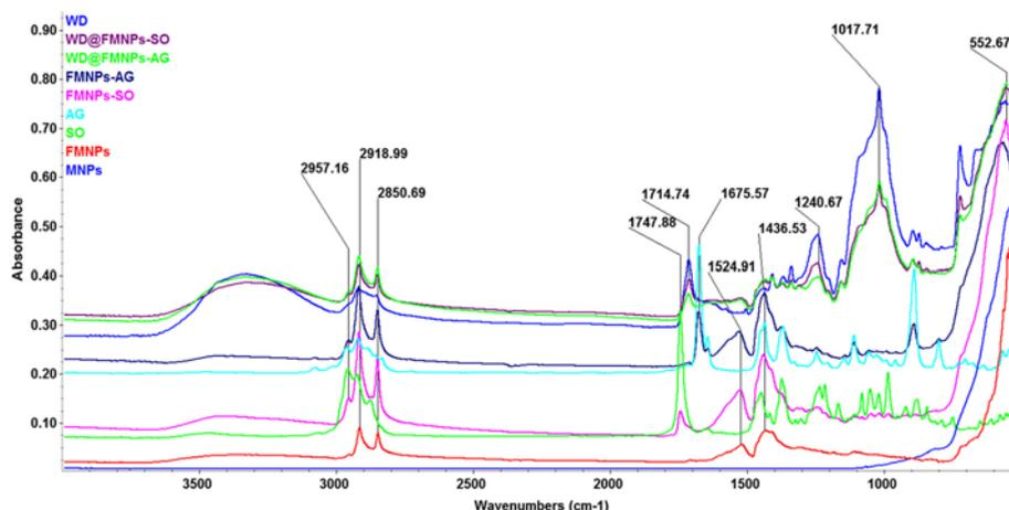
**Figure 4** FT-IR spectra of WD, WD@FMNPs-SO and WD@FMNPs-AG.
